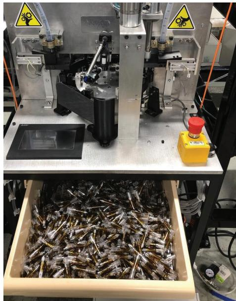
eVolve’s Raptor cartridge filling machine uses a custom Nason pump cylinder for accurate dispensing regardless of temperature or viscosity.
